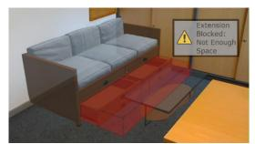
Figure 3. The system warns the user if movable parts of a piece of furniture, like a drawer, would be blocked by another object.
